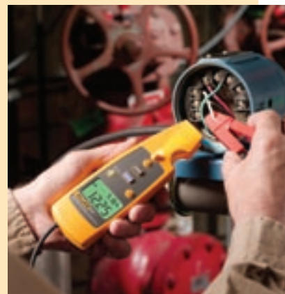
Detachable clamp used to measure 4 mA to 20 mA signals on transmitters without breaking the loop.
